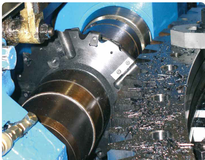
Finishing gasher with profile ground inserts Outer ring module 20; material: 42CrMo4 finishing (2nd cut)
