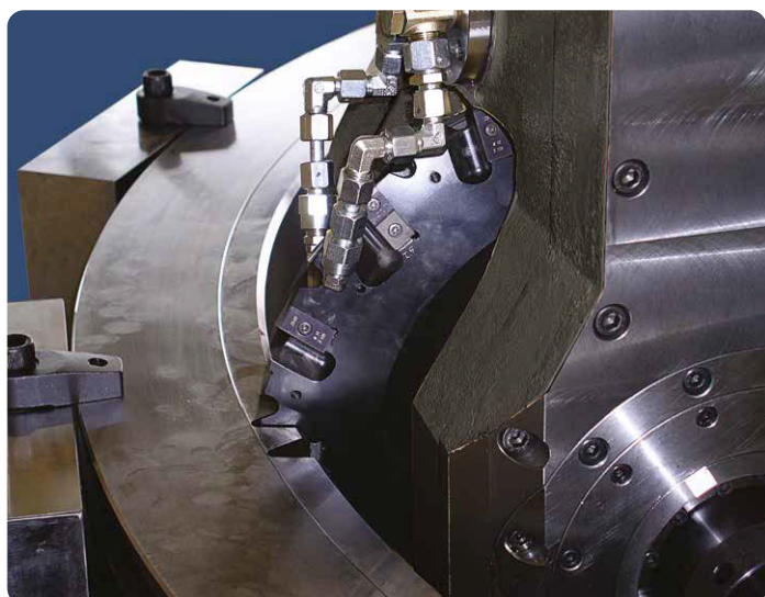
Finishing gasher with profile ground inserts Inner ring module 10; material: 42CrMo4 finishing
